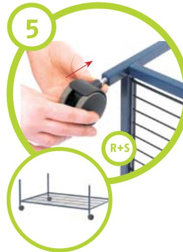
Install the 4 castors (R+S) by turning them in at the bottom of the H-shape tubes (N). The wheels with brake need to be installed at the front of the cage.
